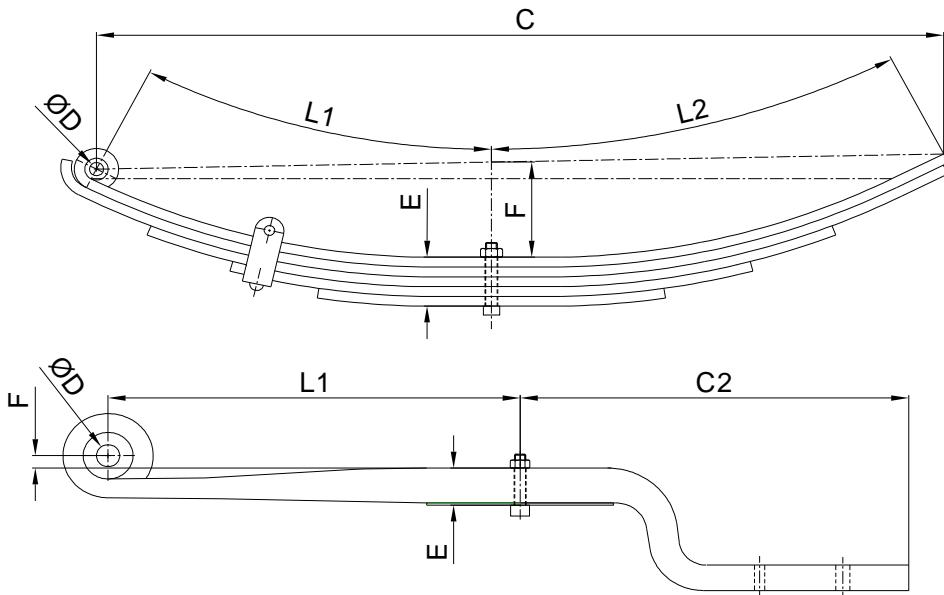
**L<sub>1</sub>** and **L<sub>2</sub>** = Length take from the middle of the eye (or end of leaf) until the C-bolt by following the leaf form.
